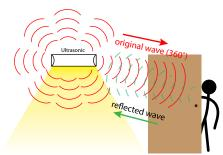
Ultrasonic motion sensors are ideal for stairwells and corridors where 360° coverage can detect motion around barriers such as staircases, workspace partitions, shelves and other obstacles in the area. Recommended for use from 8-12ft mounting
