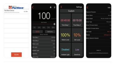
The PacWave™ Sensor mobile application complements your Bluetooth® Smart enabled PacWave™ Ultrasonic, Microwave, and PIR bi-level occupancy sensors by providing a simple user interface to configure the sensor's settings beyond what the physical controls can offer, view real-time feedback from the sensor, and control your lighting.
